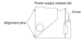
Figure 58. Controller and power supply release tabs
